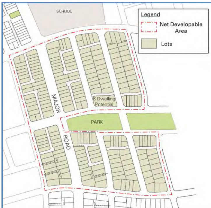
Figure 28: Example for calculating Net Residential Density of a subdivision application
