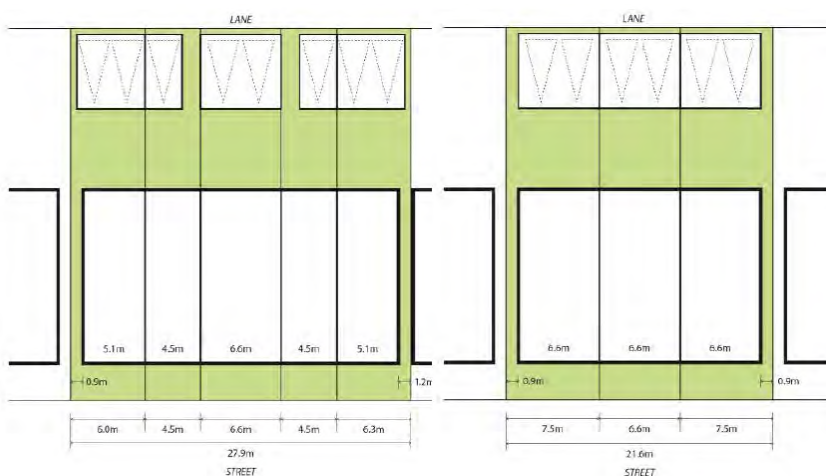
Figure 31: Two examples of lot subdivision for 'sets' of attached or abutting terraces.
