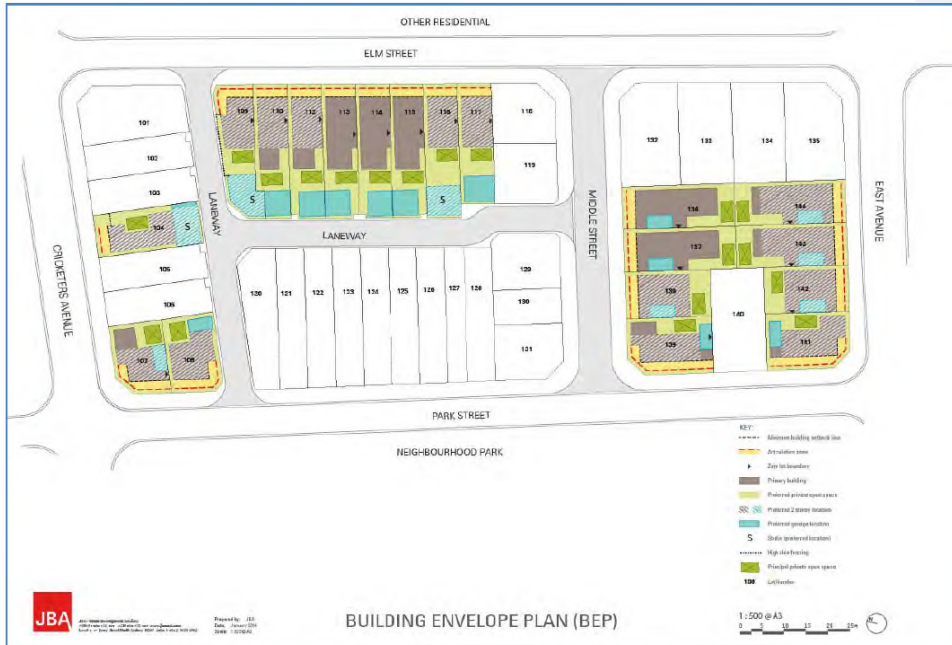
Figure 35: Sample of a Building Envelope Plan (BEP)
