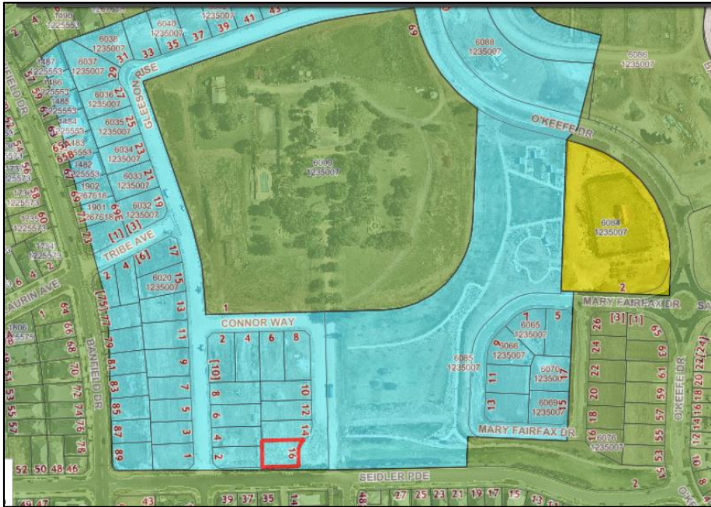
Figure 3 – Extract of Height of Building map (5m height limit shown in blue, with 9m height in green)
