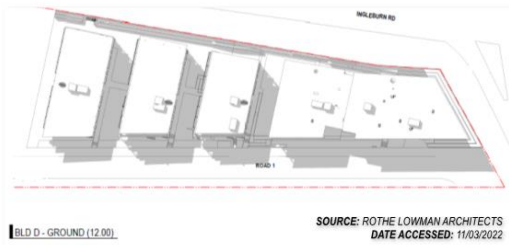
FIGURE 16: SHADOW DIAGRAM FOR 12:00PM 21 JUNE
