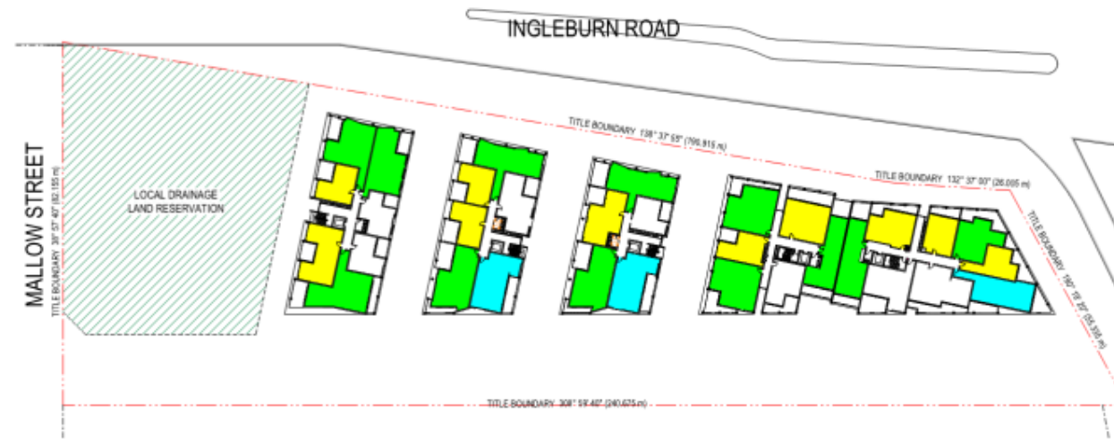
BLD-D - LEVEL 2 SOLAR / CROSS VENT
