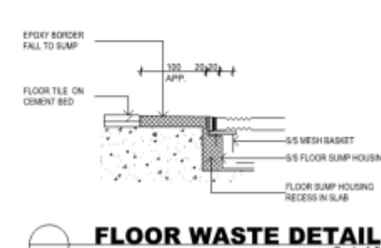
FLOOR WASTE DETAIL Scale 1:5
