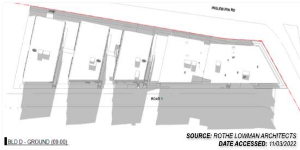
FIGURE 15: SHADOW DIAGRAM FOR 9:00AM 21 JUNE
