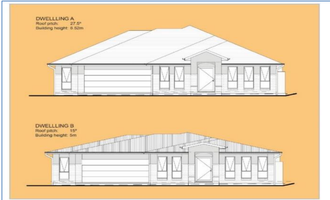
Figure 10 – Front elevation of a dwelling house with a minimum roof pitch of 15 degrees compared to a dwelling house with a minimum roof pitch of 27.5 degrees.
