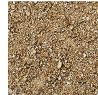
Permeable paving: Stabilised decomposed granite
