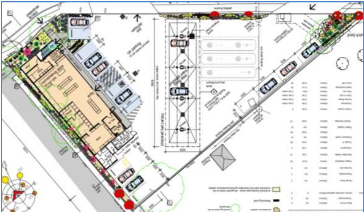
Figure 4: Extract of the approved landscaping plans. Noting the trees for retention, planting between car parking spaces 2 and 3, planting between driveways, and planting along the western boundary.
