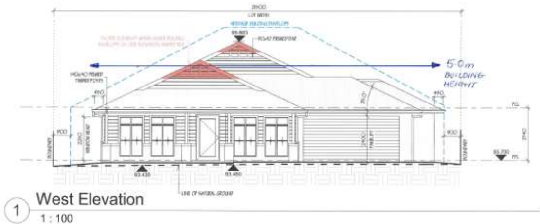
Figure 3: Proposed front elevation (red shaded gable areas relates to Heritage NSW building envelope).
