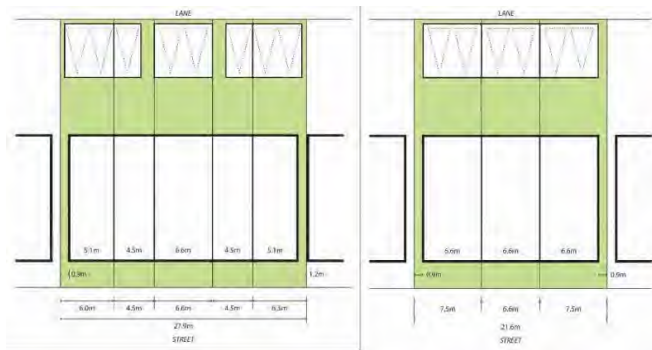
Figure 40: Two Examples of Lot Subdivision for 'Sets' of Attached or Abutting Terraces
