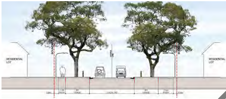
Figure 24: Hassall Driveway Cross Section
