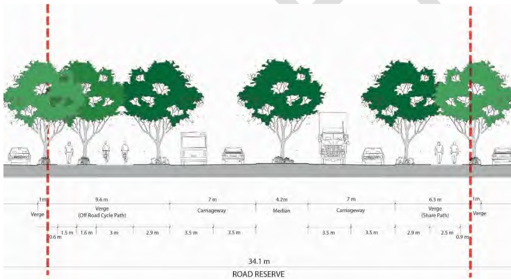
Figure 2-242425: Sub-Arterial Road Cross Section (Off-Road Cycle Lane)
