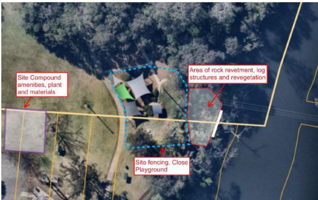
Figure 2-3 Contractor Compound and Associated Features for Site 4
