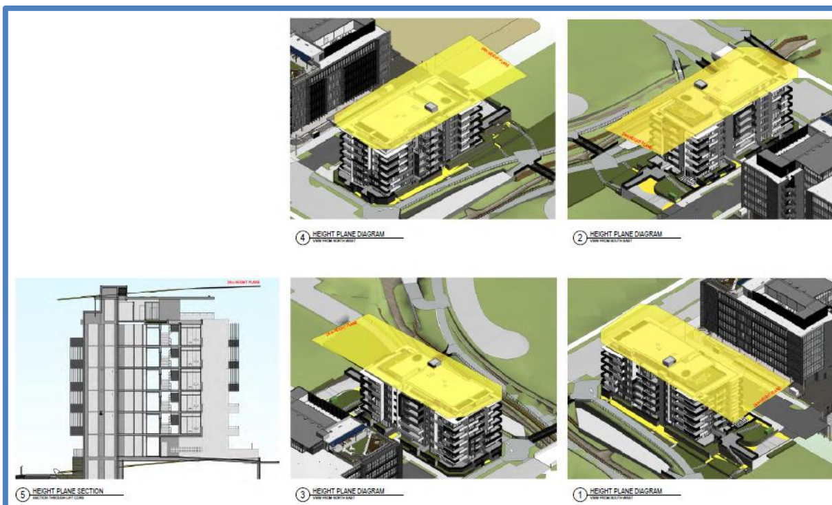
Figure 8: Building Height Planes showing no additional encroachment into 24m maximum building height.
